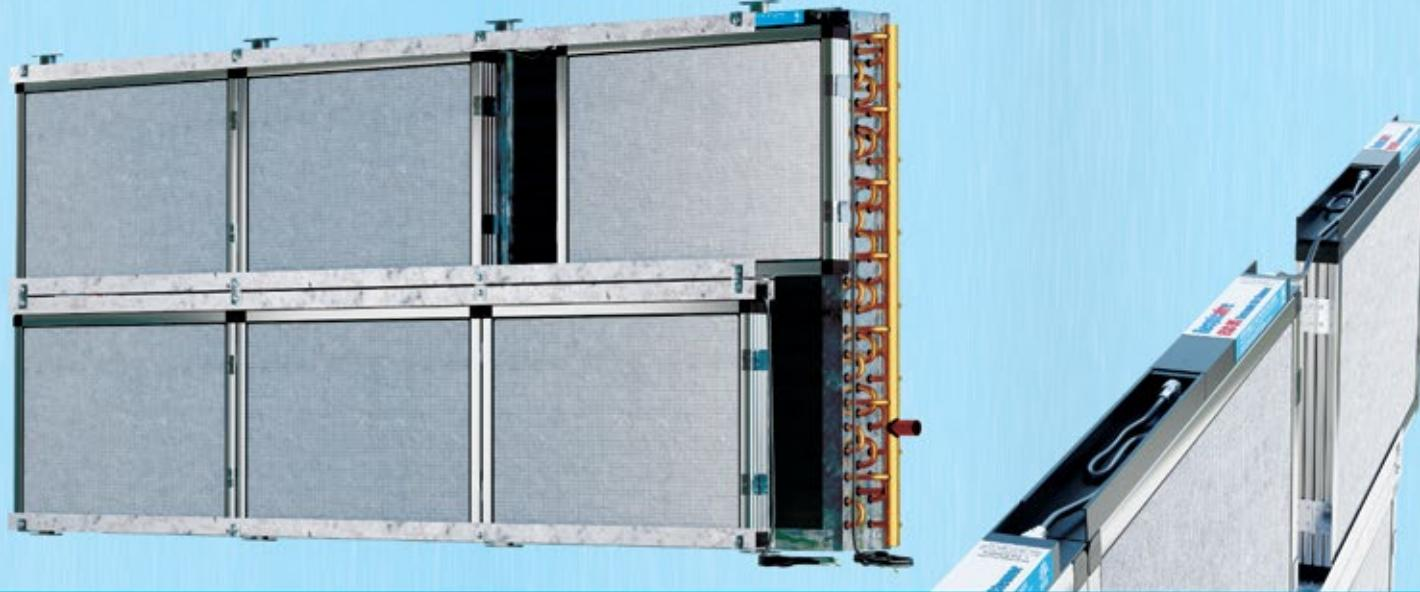
The Respicaire ECC™ 2" Polarized Media Electronic Air Cleaner is designed for the self contained filter racks inside Commercial Packaged, Rooftop & Air Handler Units. The ECC offers minimum MERV 10 and equivalent to MERV 13 filtration as indoor air recirculates through HVAC systems. It is 95% efficient on the most troublesome airborne allergens & micro particulates such as pollen, dust, dander, debris, smoke & microbes.
